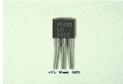
It has an output voltage that is proportional to the Celsius temperature. The scale factor is .01V/°C The LM35 does not require any external calibration or trimming and maintains an accuracy of +/-0.4 °C at room temperature and +/- 0.8 °C over a range of 0 °C
