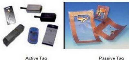
Active tags require a power source i.e., they are either connected to a powered infrastructure or use energy stored in an integrated battery. In the latter case, a tag's lifetime is limited by the stored energy, balanced against the number of read operations the device must undergo. However, batteries make the cost, size, and lifetime of active tags impractical for the retail trade. Passive RFID is of interest because the tags don't require batteries or maintenance.
