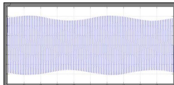
Figure 12. Fluctuating output voltage (9%-1Hz)
