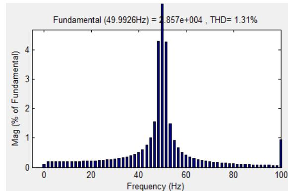
Figure 10. Spectrum of the output voltage (9%-1Hz)
