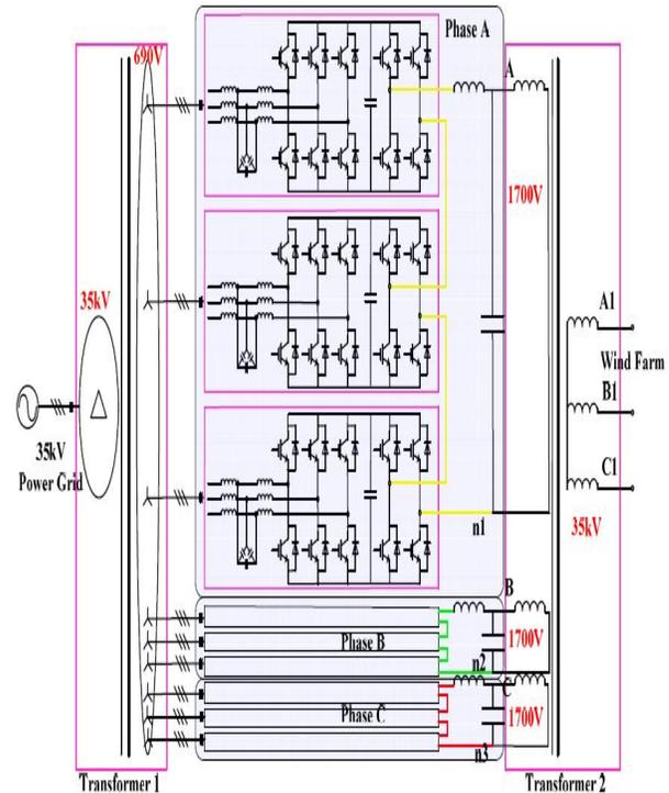
Fig. 1 Main circuit topology of the wind turbine low-frequency disturbance testing system
