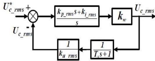
Figure 7. Control diagram of RMS outer-loop
