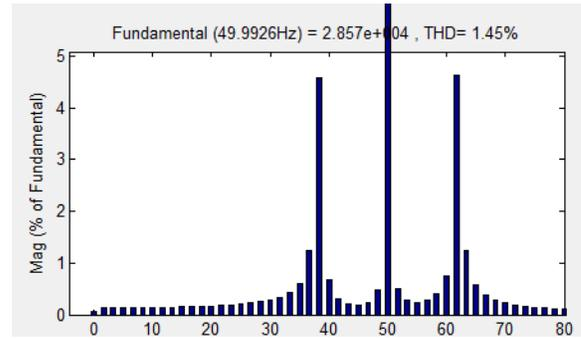
Figure 9. Spectrum of the output voltage (10%-12Hz)
