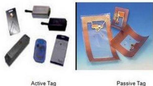
Active tags require a power source i.e., they are either connected to a powered infrastructure or use energy stored in an integrated battery. In the latter case, a tag's lifetime is limited by the stored energy, balanced against the number of read operations the device must undergo. However, batteries make the cost, size, and lifetime of active tags impractical for the retail trade.
