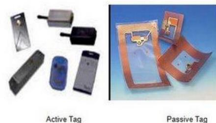
Active tags require a power source i.e., they are either connected to a powered infrastructure or use energy stored in an integrated battery. In the latter case, a tag's lifetime is packet-switched cellular technologies. It is now maintained
