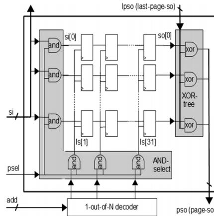
Fig 3: SCAh-page, global scan enable not shown
