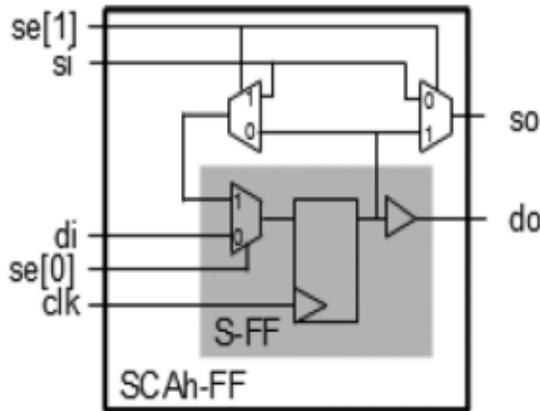
Fig 1: SCAh-FF based on an S-FF
