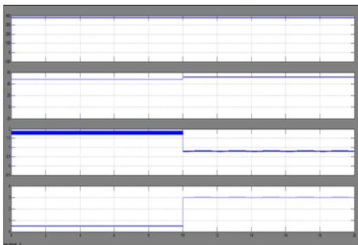
Fig. 6. Measured waveforms of mode operation in period 1  $R = 1204 \Omega$ , (Ch1:  $V_o$ , Ch2:  $V_b$ , Ch3:  $I_b$ , Ch4:  $I_{pv}$ )
