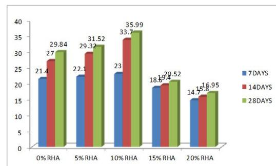
The chart shows the compressive strength of concrete at 7 days 14 days 28 days of curing period. from the
