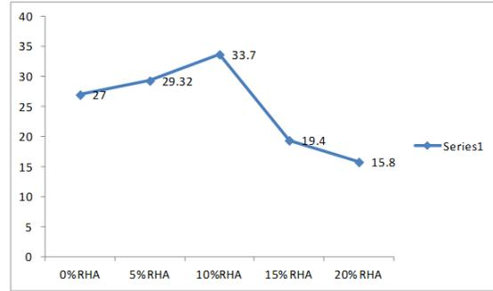
The above graph represents the compressive strength results for 14 days curing. The results shows that the strength gradually increasing with increasing in percentage of Rice husk ash. So it is advisable to use up to 10%Rice husk ash to get desired strength.
