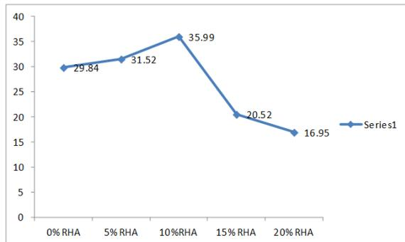
The above graph represents the compressive strength results for 28days curing. The results shows that the strength gradually increasing with increasing in percentage of Rice husk ash. So it is advisable to use up 10% Rice husk ash to get desired strength. .
