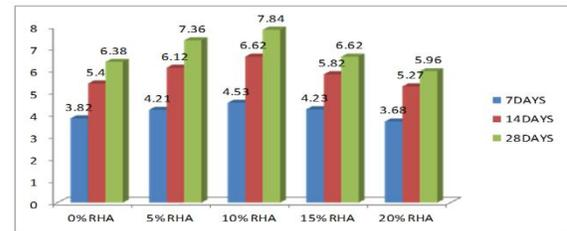
Split tensile Strength of M25 Grade Concrete with Different Percentages of Rice husk ash replacement in Normal Sand for 7 days Curing
