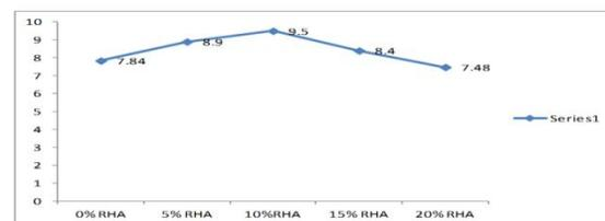
The above graph represents the split tensile strength results for 14 days curing. The results shows that the strength gradually increasing with increasing in percentage of Rice husk ash. So it is advisable to use up to 10%Rice husk ash to get desired strength.
