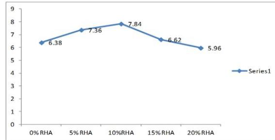
**COMPARISON OF SPLIT TENSILE STRENGTH OF MODIFIED CONCRETE**
