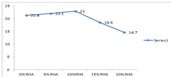
**Compressive Strength of M25 Grade Concrete with Different Percentages of replacement Rice husk ash in Normal Sand for 14 days curing.**
