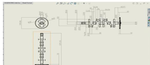
Fig.4: Dimensions of crank shaft
