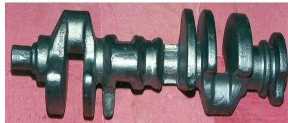
Fig.3: Crank shaft
