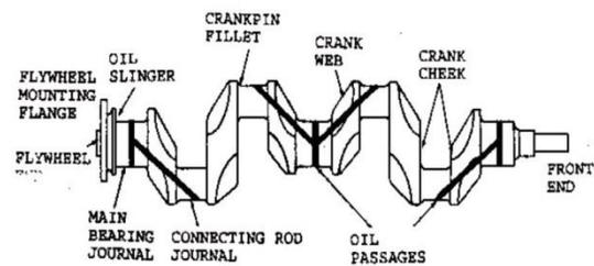
Fig1: Parts Attached To Crank Shaft
