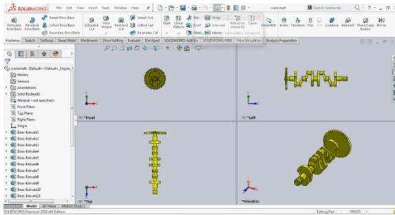
Fig.6: Four views of cam shaft
