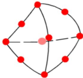
A tetrahedral element. Red dots represent nodes. Edges of an element can be curved or straight.
