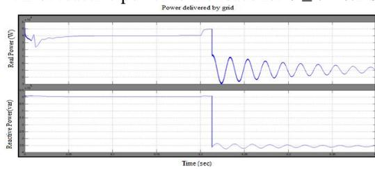
Fig. 7. Real (top) and reactive (bottom) power delivered by the grid.
