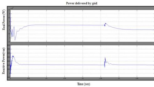
Fig. 12. Real (top) and reactive (bottom) power delivered by the grid.
