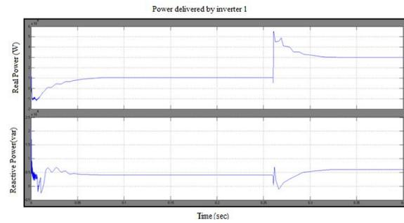
Fig. 15. Real (top) and reactive (bottom) power delivered by inverter 1.
