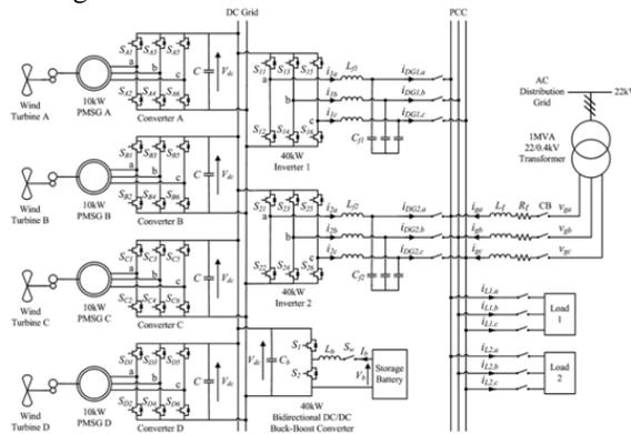
Fig. 1. Overall configuration of the proposed dc grid based wind power generation system in a micro grid.
