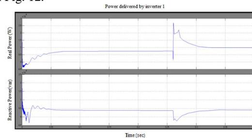
Fig. 10. Real (top) and reactive (bottom) power delivered by inverter 1.
