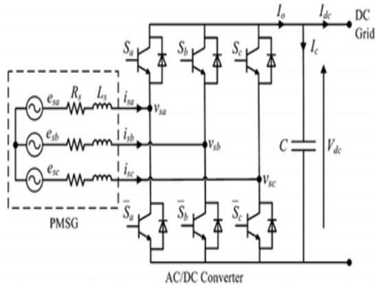
Fig. 2. Power circuit of a PMSG connected to an ac/dc voltage source converter.
