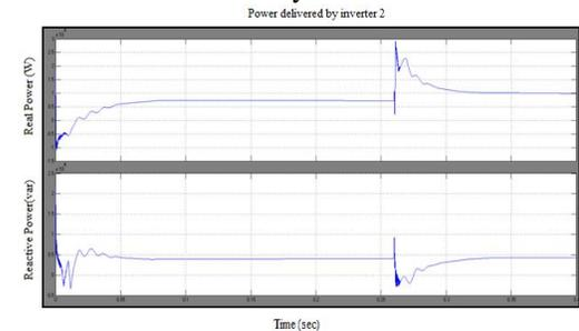
Fig. 11. Real (top) and reactive (bottom) power delivered by inverter 2
