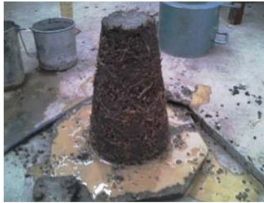
Pictorial view of the slump cone after the removal of the standard slump cone for PPFRC trial mix.
