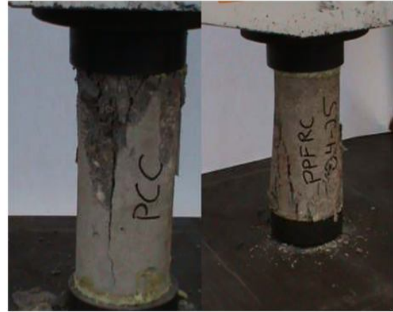
Pictorial views of PPC and PPFRC specimens under compressive strength test.
