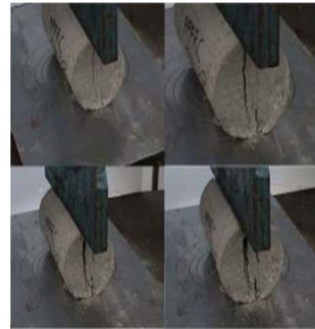
Pictorial view of crack propagation of PPERC cylinder under splitting tensile strength
