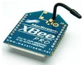
Fig 3: ZIGBEE Module
