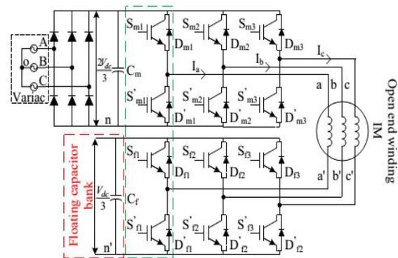
Fig. 3. Power stage of the floating bridge topology (the floating capacitor is charged to half of the main DC link voltage).
