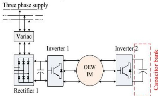
Fig. 2. Block diagram of proposed floating bridge topology.
