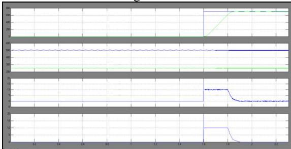
Fig. 21. FOC response of no load speed to a step reference speed command.
