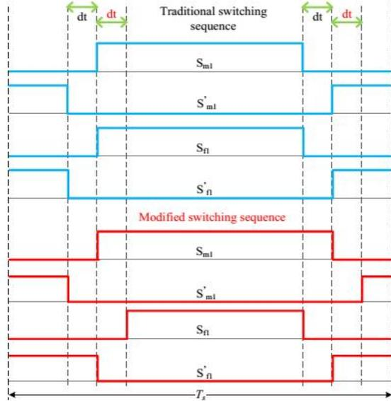
Fig. 7. Delayed dead-time intervals in both converters when current direction is positive.
