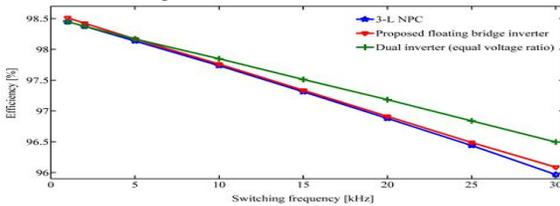
Fig. 13. Loss comparison in different power converter topologies.
