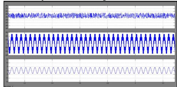
Fig. 23. Phase voltage and current under FOC when machine is loaded.
