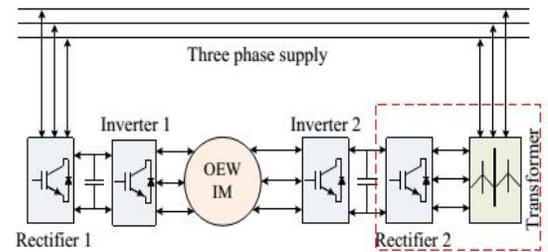
Fig. 1. Conventional open end winding IM drive topology.
