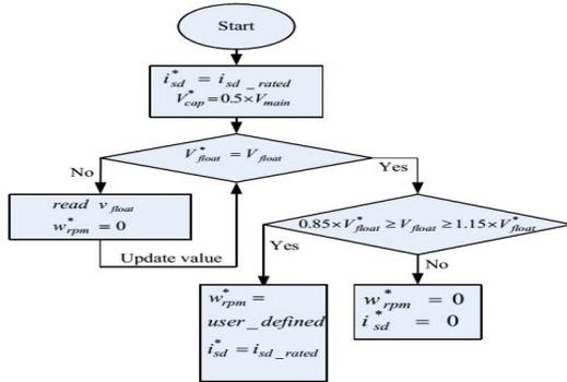
Fig. 19. Floating capacitor charging and protection algorithm
