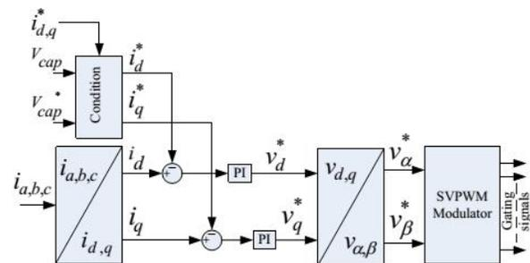
Fig. 18. Block diagram of vector control drive.
