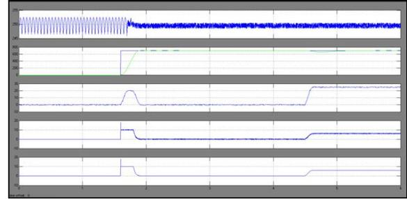
Fig. 22. FOC response to a step load applied after the speed reaches steady state.
