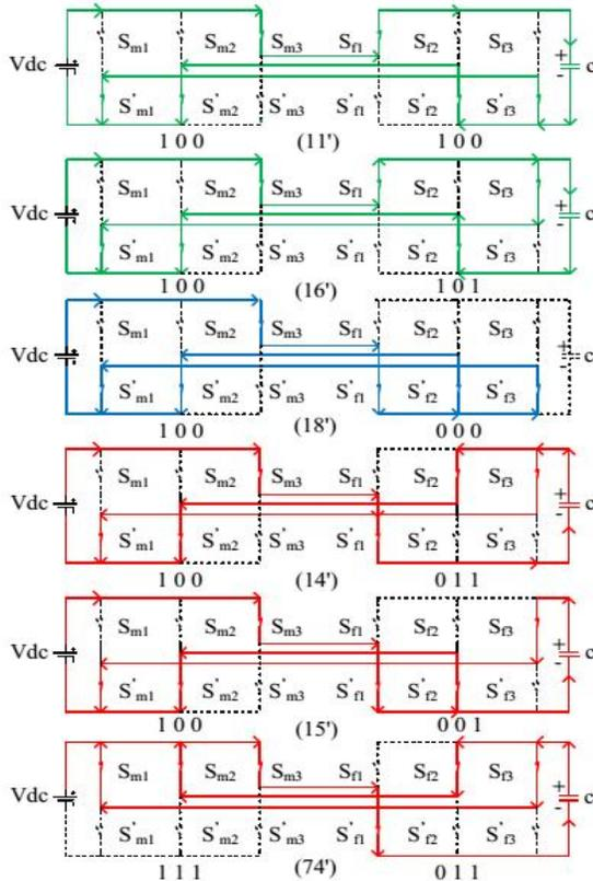
Fig. 5. Current flow for different switching state
