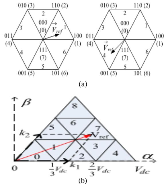
Fig. 6. (a) Space vector diagram of individual converter (not in scale). (b) Space vector diagram of the dual inverter system with source ratio of 2:1
