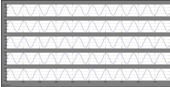
Fig. 10. Harmonic voltage amplification during a single DG unit gridconnected operation (without damping) [from upper to lower: (a) PCC voltage (THD = 4.0%); (b) node 1 voltage (THD = 4.56%); (c) node 3 voltage (THD = 10.91%); (d) node 5 voltage (THD = 12.59%); (e) DG unit filter capacitor voltage (THD = 0.38%)].
