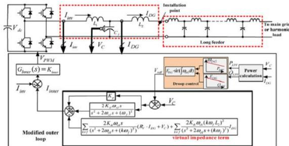
Fig. 9. Mitigation of harmonic propagation using virtual resistor and nonlinear virtual capacitor.
