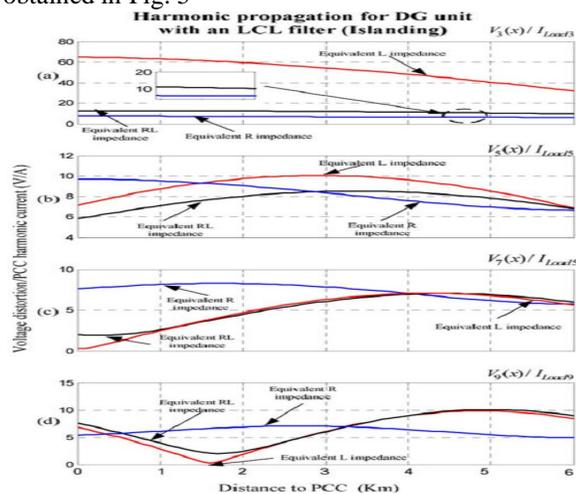
Fig. 5. Harmonic voltage amplification in a single DG unit islanding operation [(a)–(d): amplification ratio at 3rd, 5th, 7th, and 9th harmonic frequencies].
