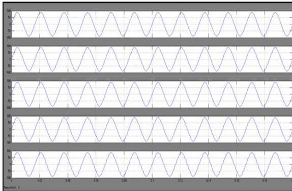
Fig. 15. Harmonic voltage amplification during a single DG unit islanding operation (with virtual nonlinear capacitor and resistor based active damping) [from upper to lower: (a) PCC voltage (THD = 6.1%); (b) node 1 voltage (THD = 6.0%); (c) node 3 voltage (THD = 5.2%); (d) node 5 voltage (THD = 5.3%); and (e) DG unit filter capacitor voltage (THD = 7.1%)].
