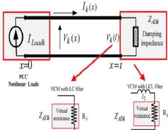
Fig. 3. Equivalent circuit of a single islanding DG unit at the kth harmonic frequency.
