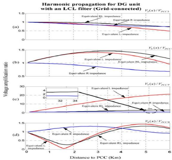
Fig. 4. Harmonic voltage amplification in a single DG unit grid-connected operation [(a)–(d): amplification ratio at 3rd, 5th, 7th, and 9th harmonic frequencies].
