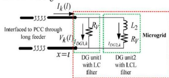
Fig. 6. Circuit diagram of a double-DG-based microgrid at the  $k$ th harmonic frequency
