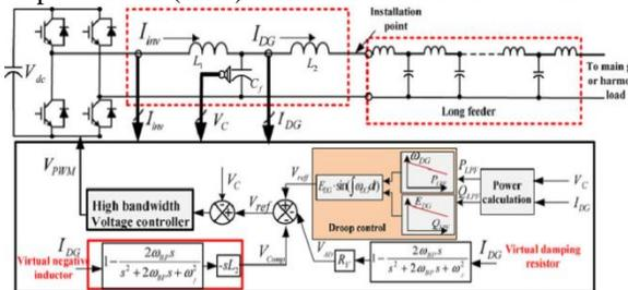
Fig. 8. Mitigation of distribution feeder harmonic propagation using virtual resistor and virtual negative inductor
