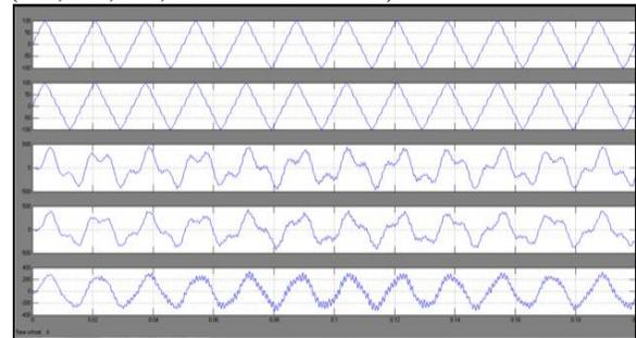
Fig. 14. Harmonic voltage amplification during a single DG unit islanding operation (without damping) [from upper to lower: (a) PCC voltage (THD = 15.2%); (b) node 1 voltage (THD = 14.7%); (c) node 3 voltage (THD = 11.9%); (d) node 5 voltage (THD = 10.5%); and (e) DG unit filter capacitor voltage (THD = 1.6%)].
