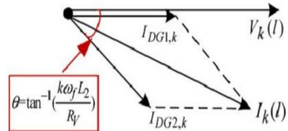
Fig. 7. Phasor diagram of the harmonic circulating current among parallel DG units.
