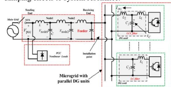
Fig. 1. Simplified one-line diagram of a single-phase microgrid service. Simulated results are provided to confirm the validity of the proposed method.
