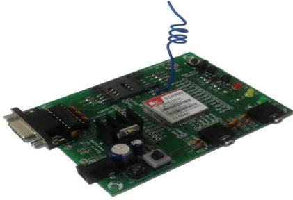
Fig 4: GSM Module
