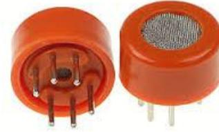
Fig 3: Alcohol sensor
