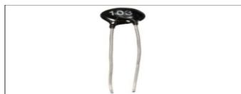
Fig 3: Temperature sensor
