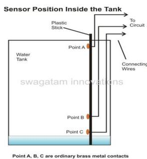
Fig 4: Water level sensor
