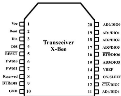
Fig 6: Zigbee pin diagram
