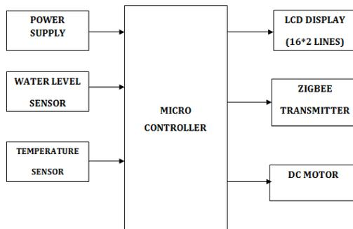
Fig 1: Transmitting section
