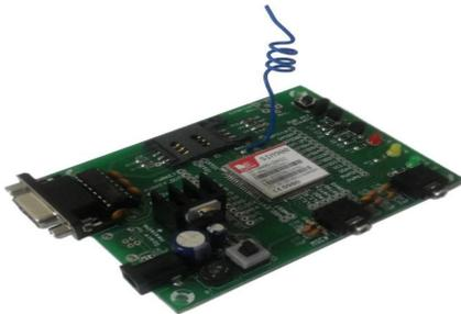
Fig 4: GSM Module
