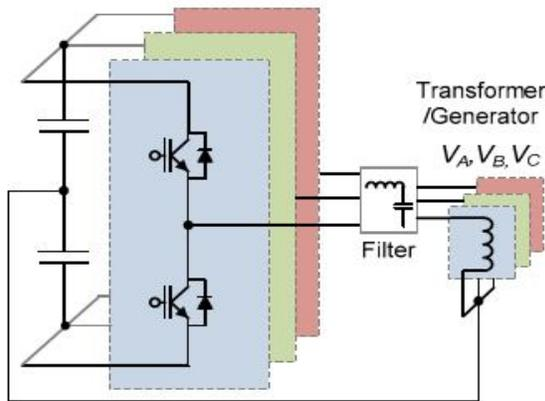
Fig. 6. Converter structure with zero sequence current path (a) Four-wire system
