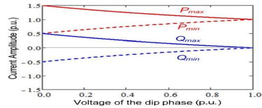
(b) P and Q oscillation range vs. VA.
