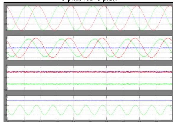
Fig. 18. Simulation of converter control with no active power oscillation and no negative sequence (three-phase converter with the zero-sequence current path,  $P_{ref}=1$  p.u.,  $Q_{ref}=0$  p.u.,  $P_{s2}=0$  p.u.,  $P_{c2}=0$  p.u.,  $i_d=0$  p.u.,  $i_q=0$  p.u.,  $V_A=0$  p.u.,  $I_+$ ,  $I_-$ , and  $I_0$
