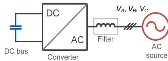
Fig. 1. A typical DC-AC converter application
