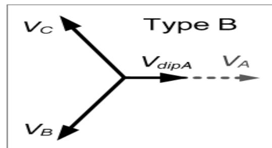
Fig. 2. Phasor diagram definitions for the voltage dips in the AC source of Fig. 1.  $V_A$ ,  $V_B$ ,  $V_C$  means the voltage of three phases in the AC source
