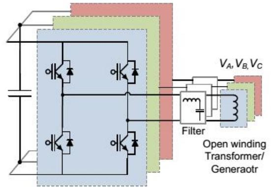
Fig. 6. Converter structure with zero sequence current path. (b) Six-wire system
