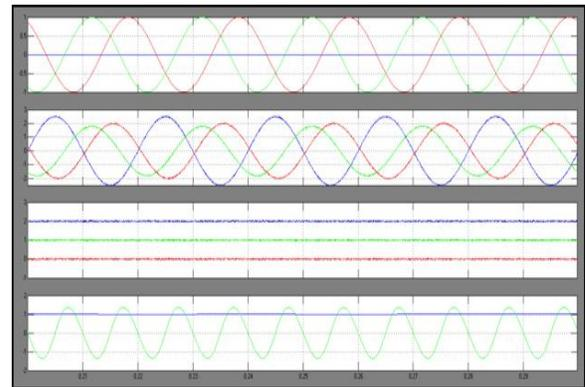
Fig. 16. Simulation of the converter control with no active power oscillation (three-phase three-wire converter,  $P_{ref}=1$  p.u.,  $Q_{ref}=0$  p.u.,  $P_{s2}=0$  p.u.,  $P_{c2}=0$  p.u.,  $V_A=0$  p.u.,  $I_+$ ,  $I_-$ , and  $I_0$  means the amplitude of the current in the positive, negative, and zero sequences, respectively).
