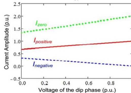
(a) Sequence current amplitude vs. VA.
