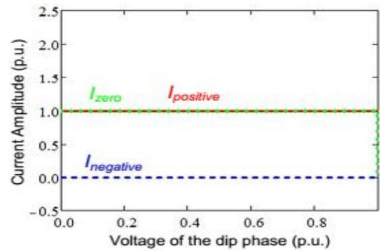
(a) Sequence current amplitude vs. VA.
