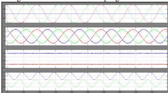
Fig. 15. Simulation of the converter with no negative-sequence current control (three-phase three-wire converter,  $P_{ref}=1$  p.u.,  $Q_{ref}=0$  p.u.,  $I_d=0$  p.u.,  $I_q=0$  p.u.,  $V_A=0$  p.u.,  $I_+$ ,  $I_-$ , and  $I_0$  means the amplitude of the current in the positive, negative, and zero sequences, respectively).
