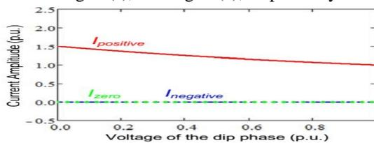
(a) Sequence current amplitude vs. VA.
