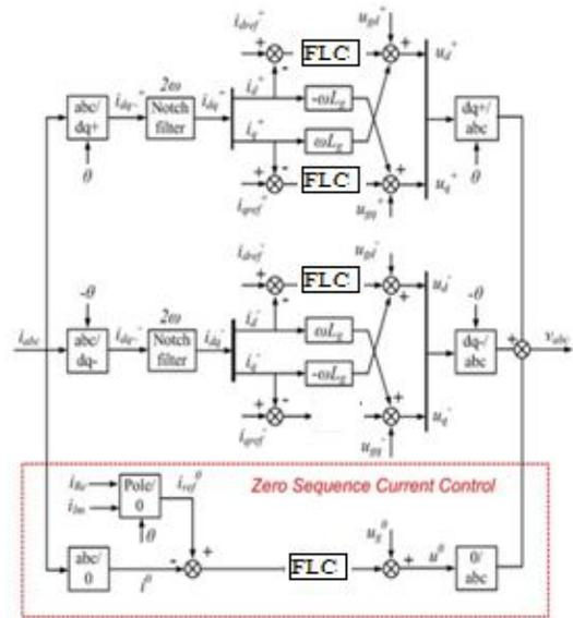
Fig. 7. Control structure for converter system with zero sequence current
