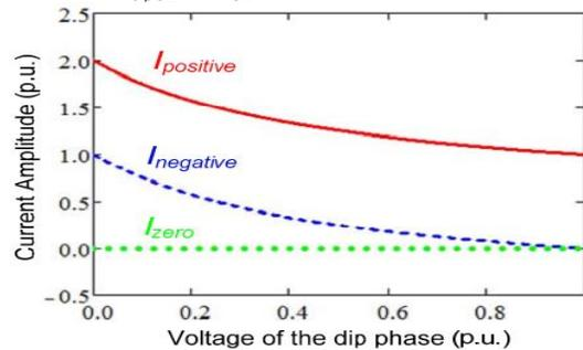
(a) Sequence current amplitude vs. VA.
