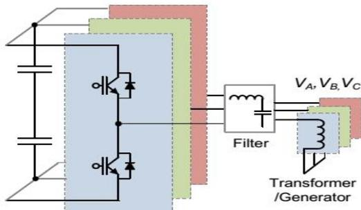
Fig. 3. Typical three-phase three-wire 2L VSC.
