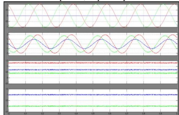
Fig. 17. Simulation of converter control with no active and reactive power oscillation (three-phase converter with the zero-sequence path,  $P_{ref}=1$  p.u.,  $Q_{ref}=0$  p.u.,  $P_{s2}=0$  p.u.,  $P_{c2}=0$  p.u.,  $Q_{s2}=0$  p.u.,  $Q_{c2}=0$  p.u.,  $V_A=0$  p.u.)
