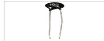
Fig 3: Temperature sensor
