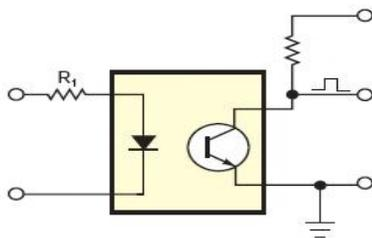
Fig 4: Optocoupler structure
