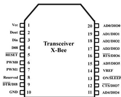
Fig 5: ZIGBEE pin diagram
