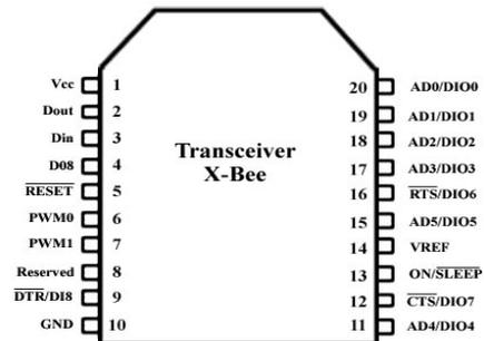
Fig 3: Pin diagram of X-Bee Transceiver
