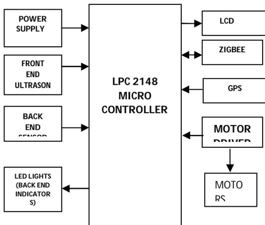
Fig.2. Vehicle 2 Monitoring Section
