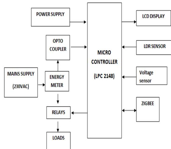
Fig.1. Field Section Block diagram
