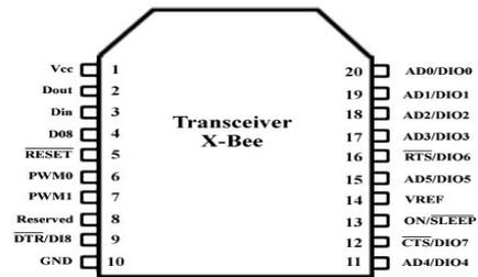
Fig 3: Pin diagram of X-Bee Transceiver
