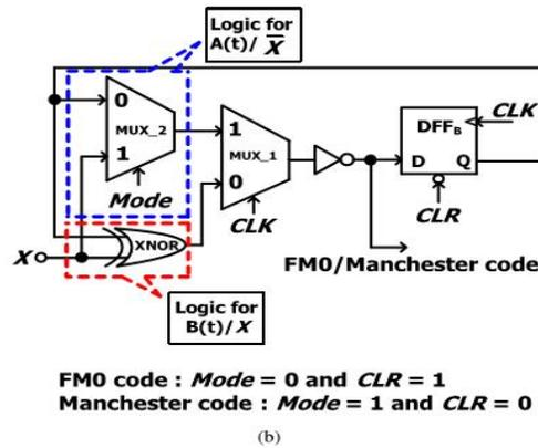
Fig. 12. VLSI architecture of FM0 and Manchester encodings using SOLS technique. (a) Unbalance computation time between  $A(t)/X$  and  $B(t)/X$ . (b) Balance computation time between  $A(t)/X$  and  $B(t)/X$ .
