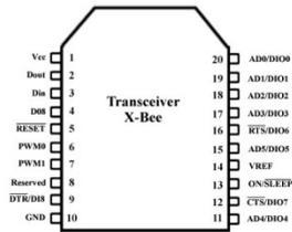
Fig 8: ZIGBEE pin diagram
