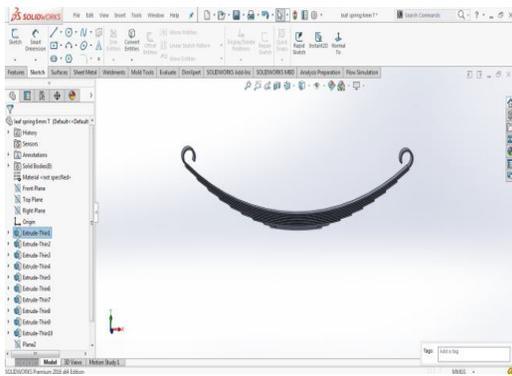
Fig 3. Leaf spring model 6mm
