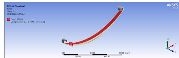
Material: carbon epoxy, thickness 6mm
