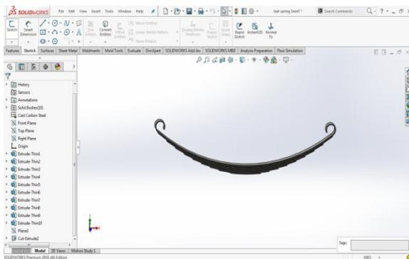
Figure4. Leaf spring model 5mm
