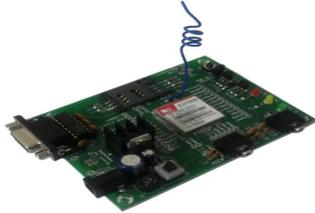
Fig 2: GSM Module
