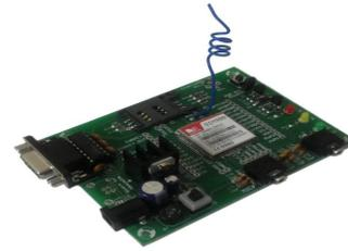
Fig 6: GSM Module
