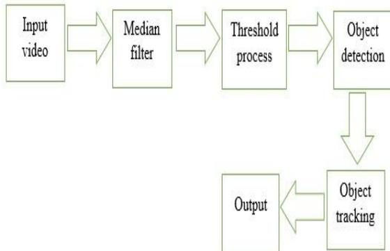
Figure 1.1: Block diagram for object detection & tracking in video
