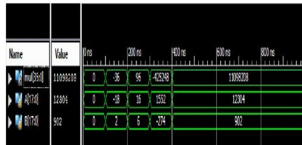
Fig. 5. Simulation Results of Booth-encoded Wallace Tree Multiplier
