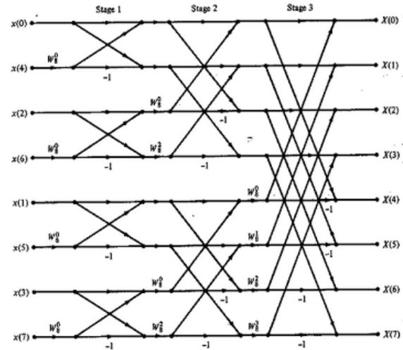
Fig. 1. Radix-2 8-point DIT-FFT algorithm
