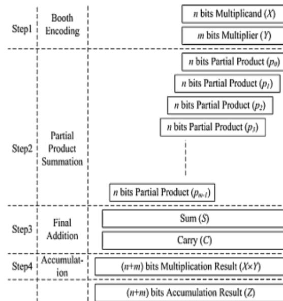
Fig. 2. Basic arithmetic steps of multiplication and accumulation.
