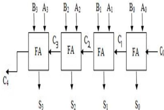
Fig. 1 4-bit Ripple Carry Adder
