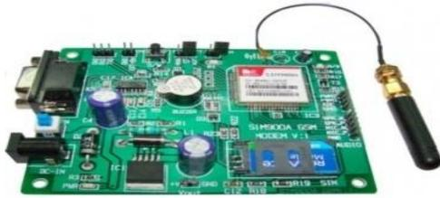
**Fig 3: GSM module**
