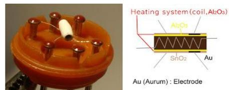
SnO<sub>2</sub> ceramics will become the semi-conductor, so there are more movable electrons, which means that it is ready to make more current flow when the alcohol molecules in the air meet the electrode that is between alumina and tin dioxide, ethanol burns into acetic acid then more current is produced. So the more alcohol molecules there are, the more current we will get. Because of this current change, we get the different values from the sensor.
