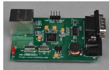
Fig 3: Ethernet module
