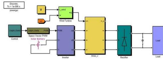
Figure 3. Simulation model of the novel wind and solar hybrid power generation systems.
