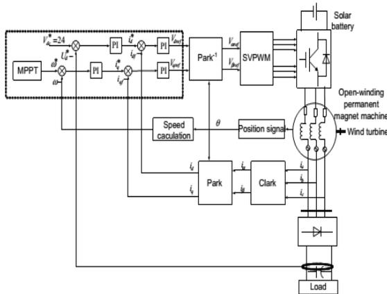
Figure 2. System control block diagram.
