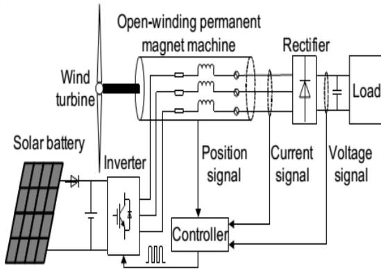
Figure 1. Structure diagram of the novel wind and solar hybrid power system
