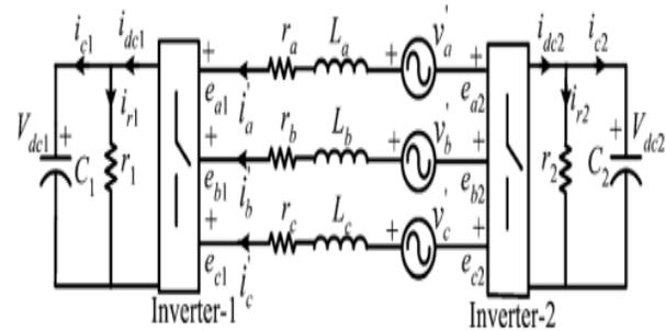
Fig. 3. Equivalent circuit of the cascaded two-level inverter-based multilevel STATCOM
