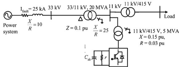
Fig. 1. Power system and the STATCOM model.
