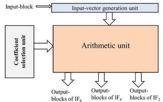
Fig. 3. Proposed reconfigurable architecture for a set of interpolation filters of up-sampling factors
