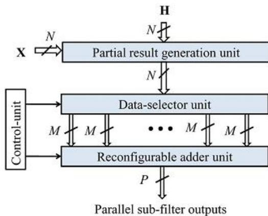
Fig. 1. Full-parallel reconfigurable interpolation filter structure where partial results are shared
