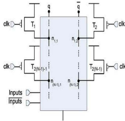
Fig. 3. Dual-switch generic scheme for N-depth DPDN.
