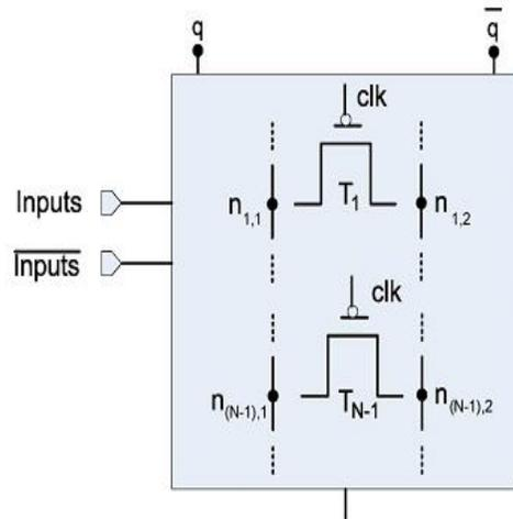
Fig. 2. Single-switch generic scheme for N-depth DPDN
