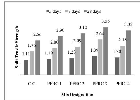
Figure: 4 Split tensile strength values of C.C and PFRC at 3, 7 and 28 Days
