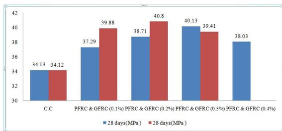
Figure: 1 Compressive strength values of C.C PFRC and GFRC 28 day
