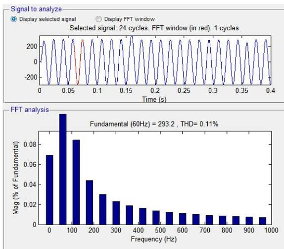
Fig11: THD Level When Five Level Diode Clamped Based Inverter is used during Voltage Sag
