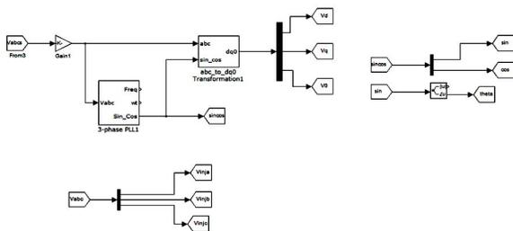
Fig .6 Controller Implementation of Dynamic Voltage Restorer
