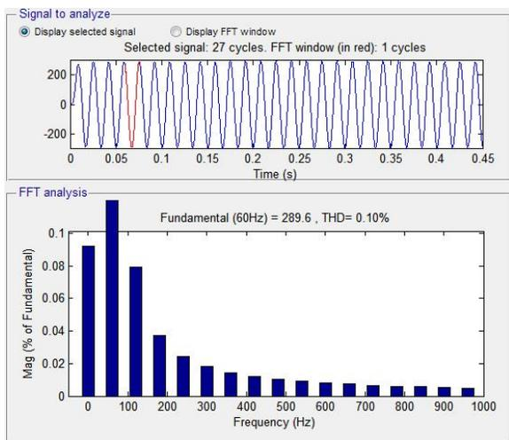
Fig 12: THD Level When Five Level Diode Clamped Inverter is used during Voltage Swell
