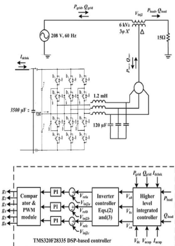
Fig. 2. Model of three-phase series inverter (DVR) and its controller with integrated higher order controller.
