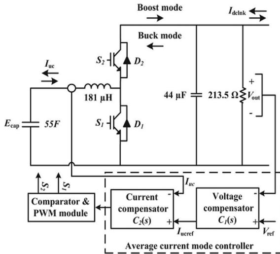
Fig. 3. Model of the bidirectional dc–dc converter and its controller.
