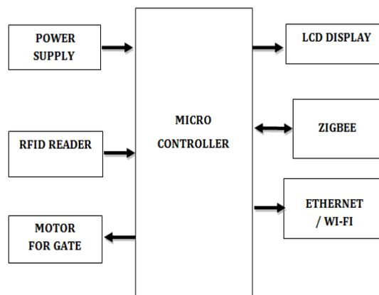
Fig 1: Security Section Block Diagram
