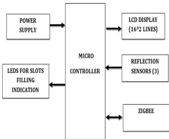
Fig 2: Parking Section Block Diagram
