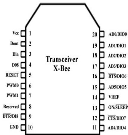
Fig 5: Pin diagram of X-Bee Transceiver
