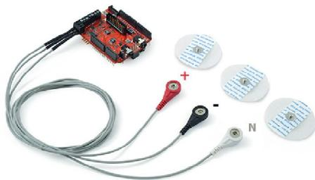
Fig 8: ECG Sensor
