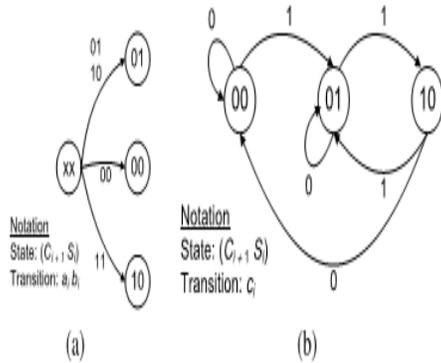
Fig. 3. State diagrams for PASTA. (a) Initial phase. (b) Iterative phase
