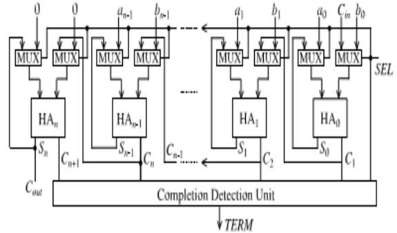
Fig. 2. General block diagram of PASTA
