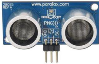
Fig: Ultrasonic sensor
