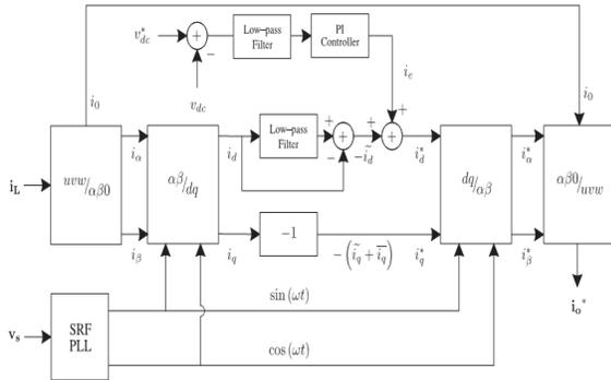
Fig. 4. DQ- Based Current Reference Generator Block Diagram.
