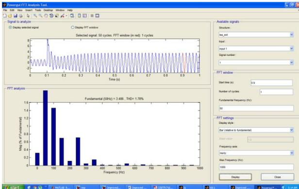
Fig14: FFT analysis of the source current after APF connection
