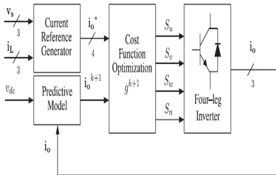
Fig.5. Proposed Predictive Digital Current Control Block Diagram.
