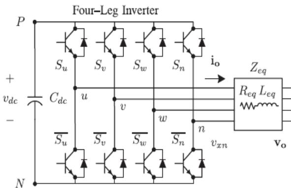
Fig.3. Two-level four leg PWM-VSI topology
