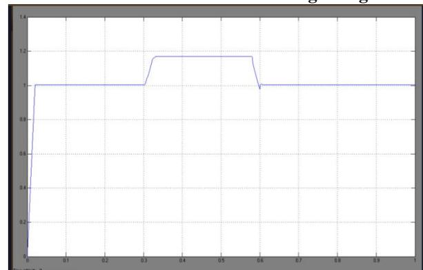
Figure 4.7: Voltage Waveform due to loss of load without D-Statcom
