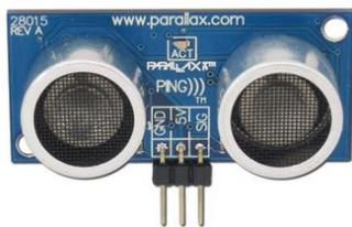
Fig: Ultrasonic sensor
