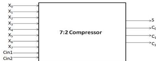
Fig. 6 Black box representation of a 7:2 Compressor Adder
