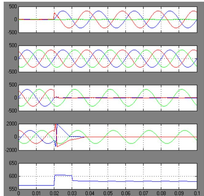
Fig. 9. (a) Injected voltages. (b) Source voltages. (c) Load voltages. (d) Line currents. (e) DC-link voltage, during the phase-to-phase downstream fault.
