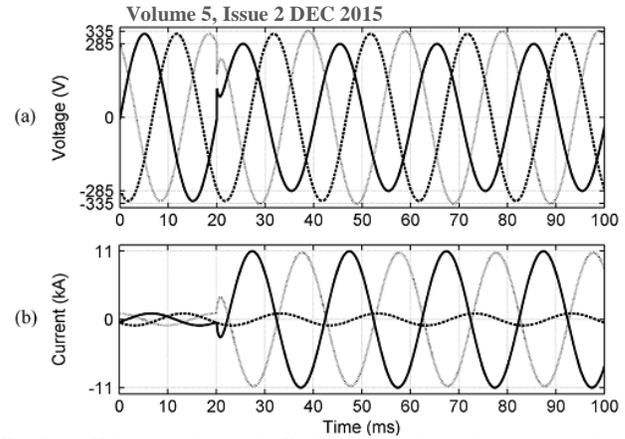
Fig. 8. (a) Voltages at bus<sub>3</sub>, (b) Fault currents, during downstream phase-to-phase downstream fault when the DVR is inactive (bypassed).
