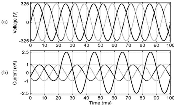
Fig.10. (a) Voltages at Bus<sub>3</sub> (b) Fault currents, during the downstream singlephase-to-ground fault when the DVR is inactive (bypassed).
