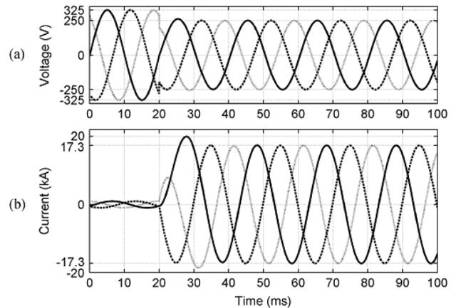
Fig.6. (a) Voltages at bus<sub>3</sub> (b) Fault currents, during downstream three-phase fault when the DVR is inactive (bypassed).
