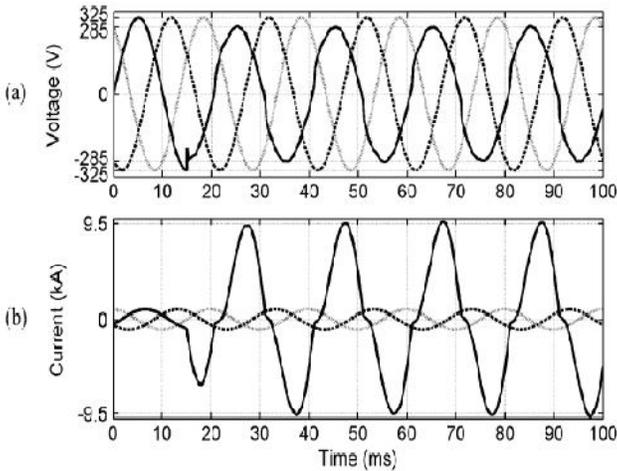
Fig.12. (a) Voltages at Bus<sub>3</sub> (b) Fault currents, during the downstream single phase-to-ground arcing fault when the DVR is inactive (bypassed).
