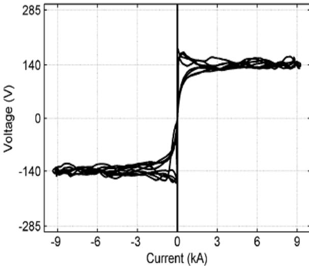
Fig. 13. Nonlinear v-i characteristic of the arc.
