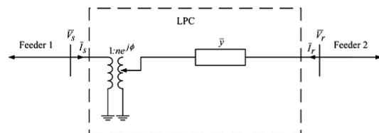
Fig.3. Circuit model of loop power controller.
