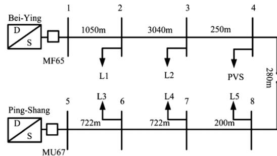
Fig.6. Taipower distribution feeders for computer simulation.
