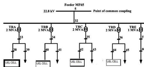
Fig. 7. One-line diagram of Kaohsiung Main Stadium.
