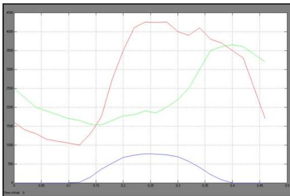
Fig. 9. Power profiles of Feeder MF65 and MU67 (with fuel cell system)
