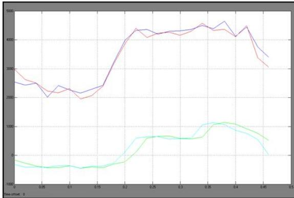
Fig. 11. Loading balance of both feeders with the control of LPC (with fuel cell system).
