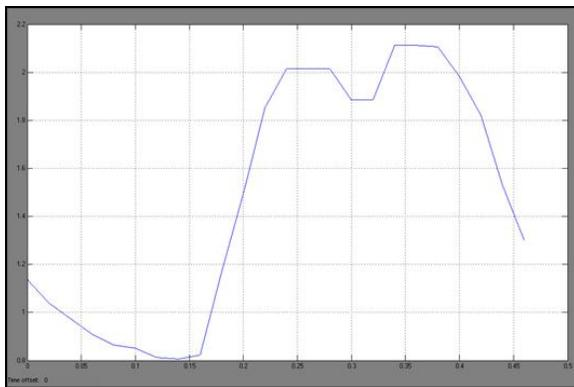
Fig. 12(a). Percentage of system power loss before applying LPC for loading balance (with fuel cell system).
